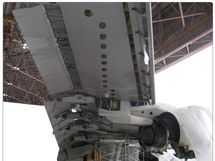
Picture 5 - A380 wing undergoing inspection
